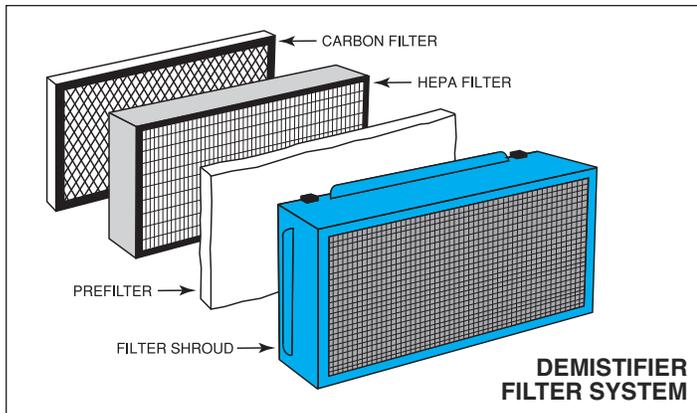
The prefilter is positioned in front of the HEPA filter and is designed to capture larger airborne particles, thereby extending the life of the HEPA filter. The carbon filter is then placed behind the HEPA to help absorb odors and vapors.
